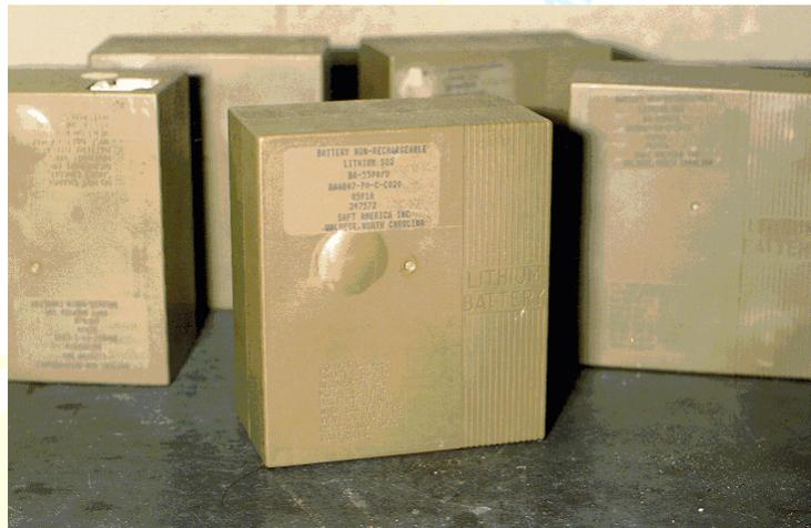
**Figure 4 Normal Battery Deformation During Discharge**
