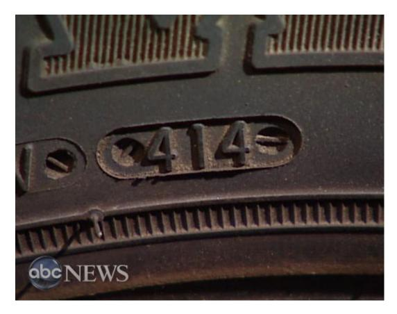
This tire's DOT code indicates that it was made in the 41st week of 1994. Tires made in the 1990s have three numbers at the end of the DOT code, while tires made after 2000 have four numbers.
