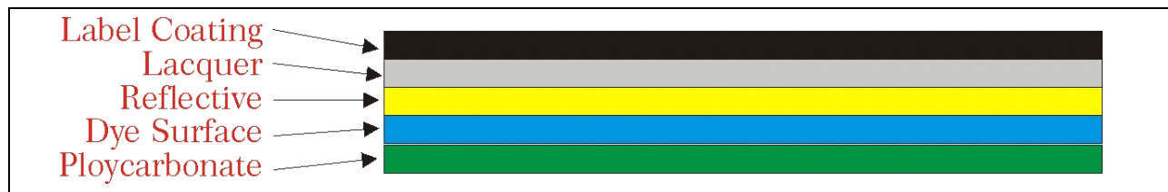
Figure 2-4. Five-layer structure of recordable discs.
