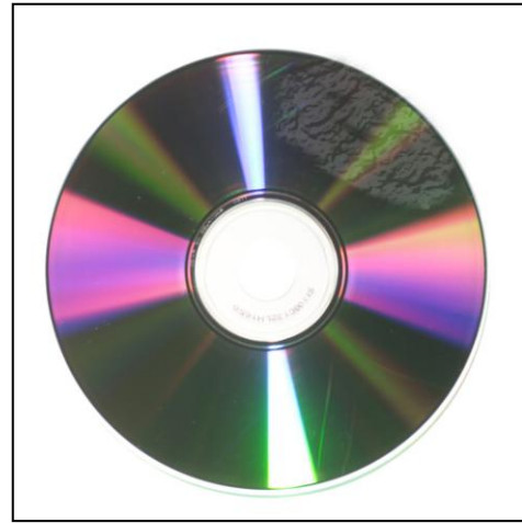
Figure 2-7. CD rot in upper right.
