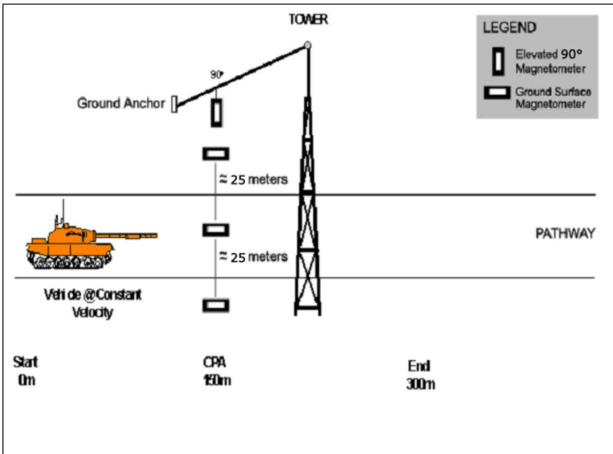
Figure 2-2. Magnetometer scenarios for a vehicular test track.
