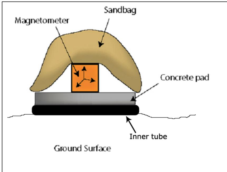
Figure 2-1. Magnetometer placement on the ground surface.
