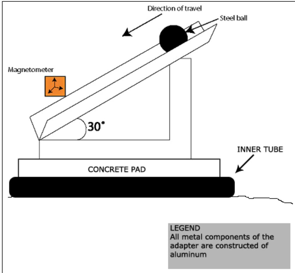
Figure 3-2. Field relative data operational checkout device.
