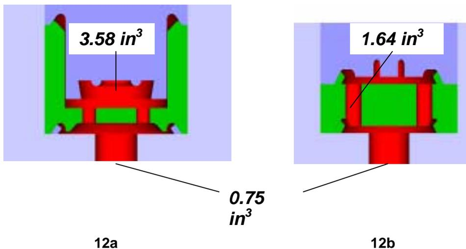
Fig. 12a: Dead volume of arrangement 6203+ 6555A
