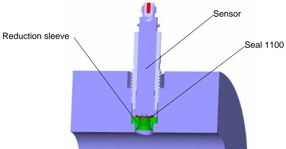
Fig. 13 Type 6215 fitted with reduction sleeve type Z14998
