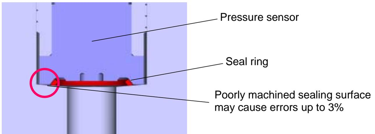
Fig. 9 concave sealing surfaces
