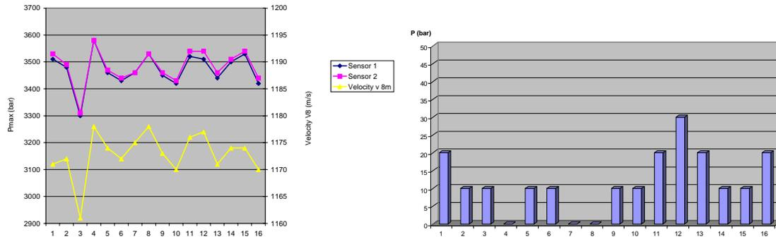
Fig. 8 Left: sequence of pressure versus velocity Right: difference between two sensors of each pair
