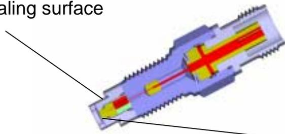
Diaphragm cavity for thermal protective plate
