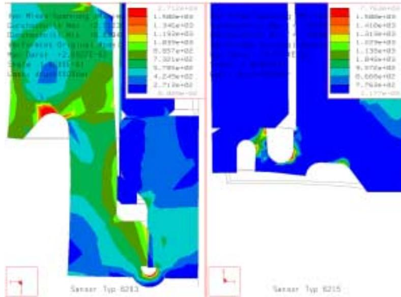
Fig. 6 (left) : The FE calculation of 6203 shows a very high loads over  $200,000\text{lb}/\text{in}^2$  at the sealing grooves and some deformations caused by the non-uniform load distribution across the entire front portion.
