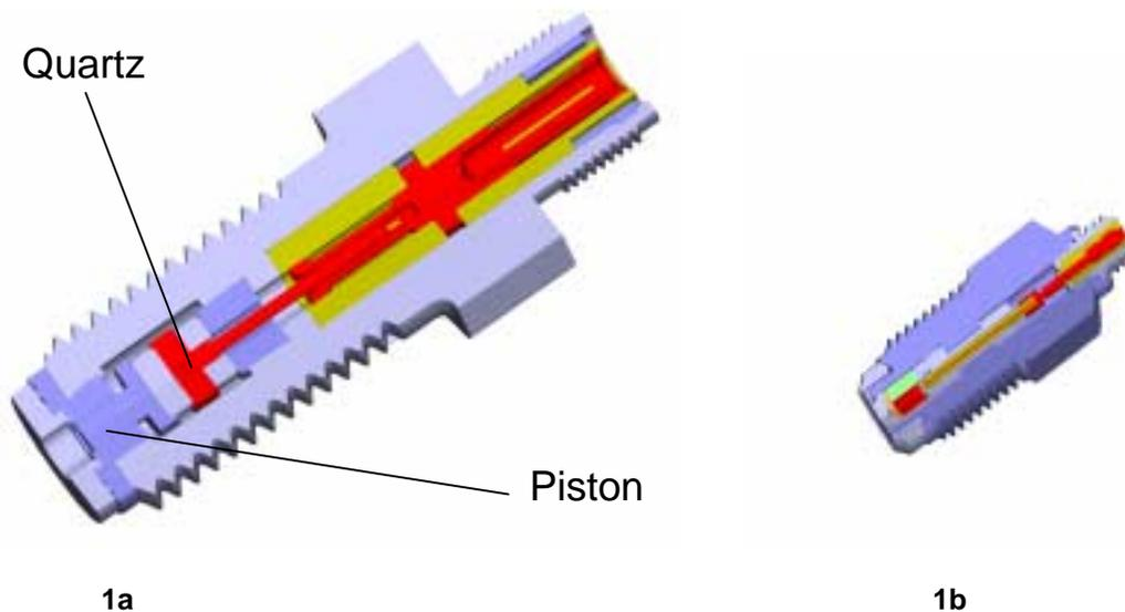
Fig. 1a transducer with piston, 24 mm thread
