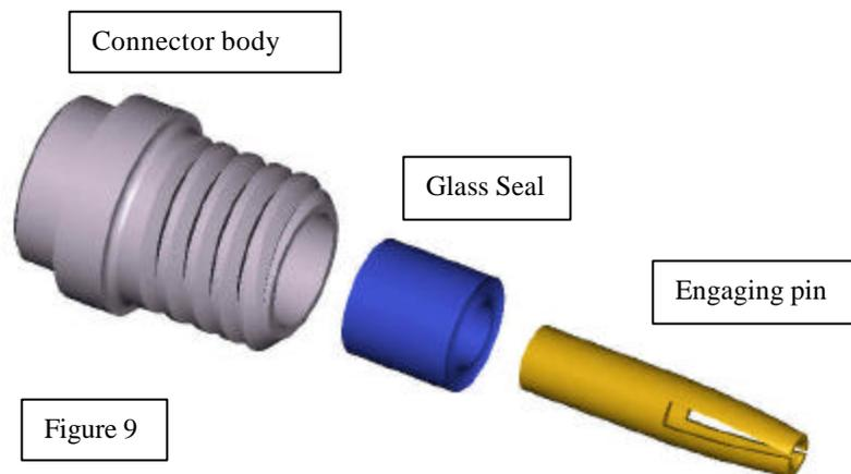
Under shock, a momentary loss of continuity with the power supply often occurs partially cutting off the event to be measured. This problem is the engaging pin material fatigue. The high temperature process involved in manufacturing the glass sealed connector reduces the stiffness of the pin material causing pin enlargement.
