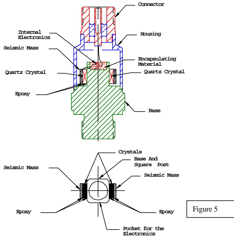
This epoxied element was a starting point toward a final solution for a quartz shock shear sensor. The engineering was quite correct because the construction limited the number of interfaces, the number of parts, and ultimately the weight of the seismic mass.
