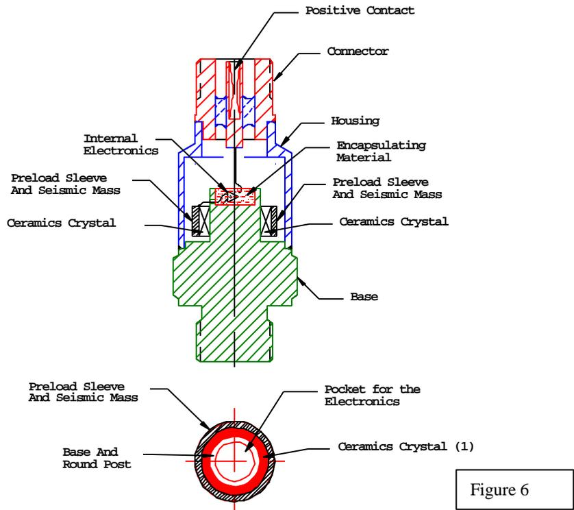
This design also lends itself to a smaller physical size. This accelerometer has been providing useful information in shock measurements up and above 100,000g's, and is well respected for its superior performance.
