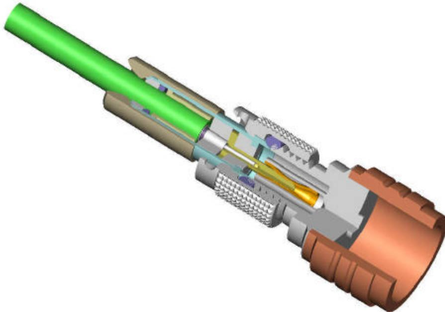
Also note that coaxial connector shown as above does not require the addition of shrink tubing to strain relieve the cable. This concept includes several mechanical-clamping mechanisms that preclude breakage. This construction minimizes the whipping effects that cause measurement errors. Figure 14 shows this improved cable-connector design compared to a conventional cable.
