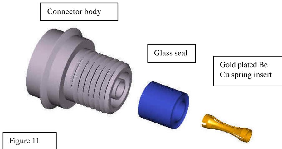
To further improve and maintain a positive connection under shock measurement conditions, an improved connector coupling design is needed.
